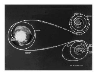
At the proper time, while behind the Moon, the CSM motor was fired giving the necessary velocity to escape Moon's gravity and get routed back to the Earth.
